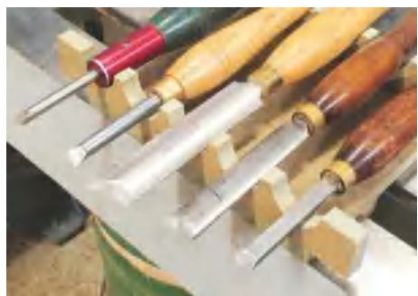
▲ Pic.1 The skew is often seen as the bad boy of turning because it is difficult to master but well worth persevering with. There are many different types, as shown here
